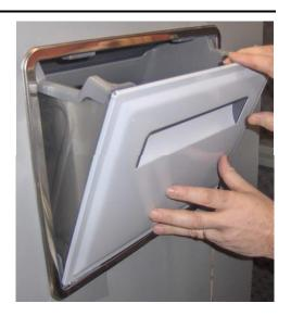
4. Remove the plastic inner container for cleaning
